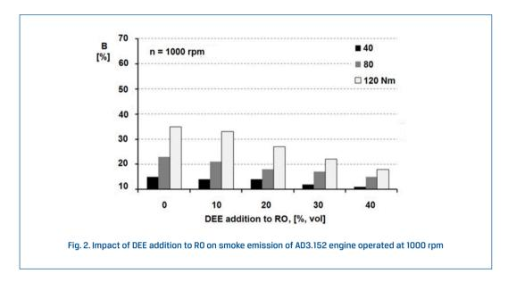
Fig. 2 presents variations of smoke opacity of AD3.152 engine operated at 1000 rpm. The engine was fuelled with RO and its blends with DEE.
