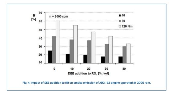
Based on the analysis of Fig. 4, it can be concluded that the smoke emission of the engine running at the speed of n = 2000 rpm is significantly higher than the results obtained at the speed of 1000 rpm. Nevertheless, it was noticed that the DEE additive reduces the exhaust smoke of the engine operating at all tested load conditions. Particularly beneficial
